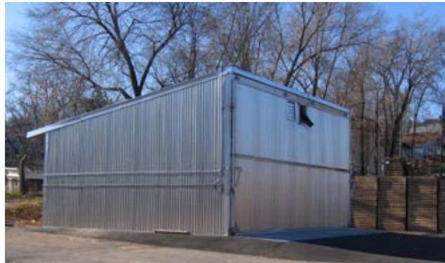
Heat Treatment Chamber treats up to 500 pallets at a time, and reaches a temperature of 220 degrees.
